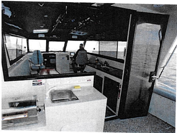
Above: The saloon offers wide-open space with lots of light and ventilation. Besides the huge windows, it has hatches in the roof top, and a large hopper window and glass cabin door opening to the cockpit.
